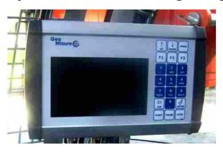
**CFA VISION** measurement system is a new generation read-out and sensor device for the drilling and grouting parameters analysed with the technology of continual auger device based on Windows CE unit with a 7" color display.
