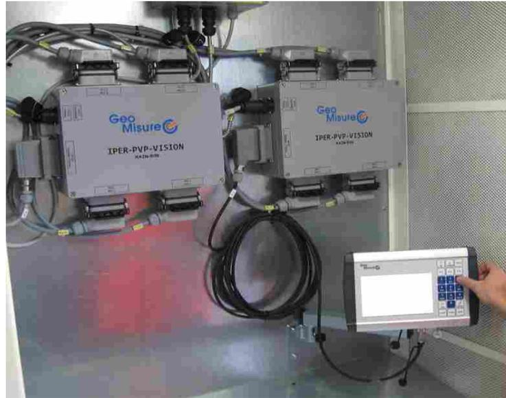
**IPER-PVP-VISION** is a system for the measuring, storage and control in the soil consolidation process with concrete injections; the system can control up to a max of 8 injectors.
