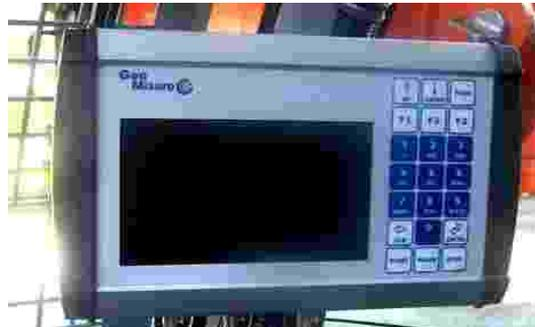
**MIX-VISION** measurement system is a new generation device used for the drilling and grouting parameters in the technology of soil mixing. It is based on Windows CE unit with a 7" color display. The system allows to measure and store the following parameters:
